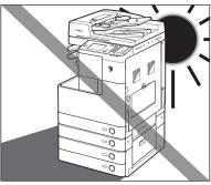
Avoid installing the machine in direct sunlight.
